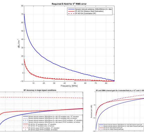
**DF Sensivity Analysis** BW = 1Hz, Receiver NF = 6dB, Max WB = 1% (Error > 45°)
